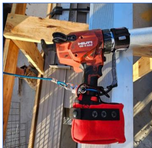
Post incident: tether designed to capture all components of the tool.
